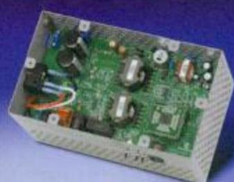
Microchip's Digital Power Interleaved PFC Reference Design
